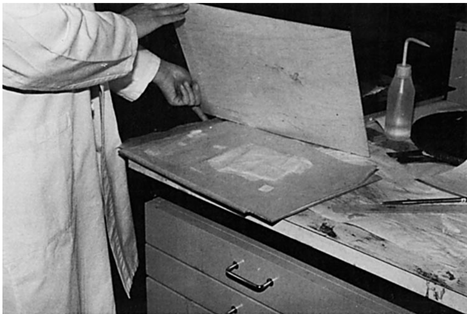
Figure 8 Removal of sample after pressing.
