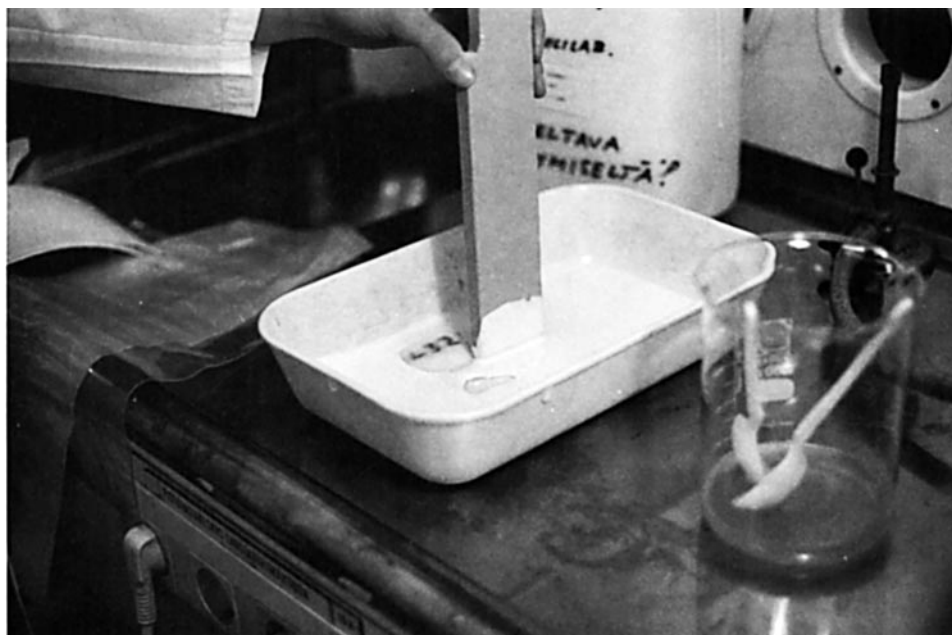
Figure 5 Latex impregnation into reinforcement mat.
